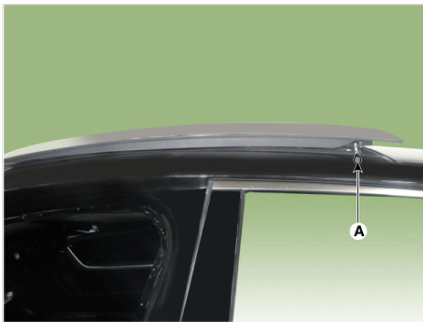
4. Carefully lift up the moving glass (A) and then remove it.
